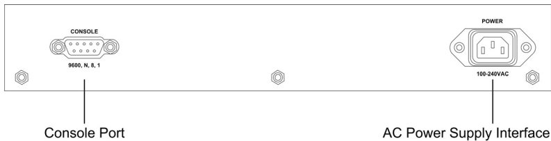
Figure 2-4. PowerConnect 2816 Back Panel
