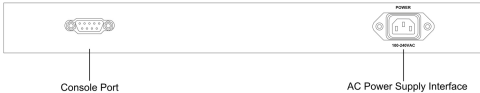
Figure 2-8. PowerConnect 2848 Back Panel
